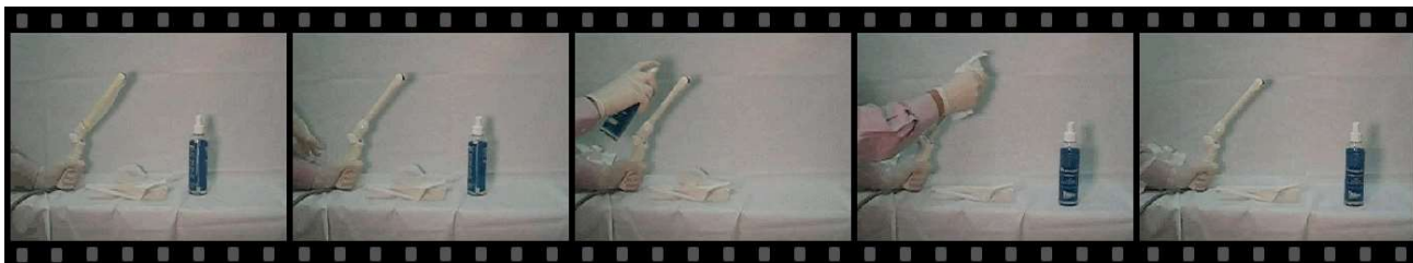
Removing cover and cleaning transducer
